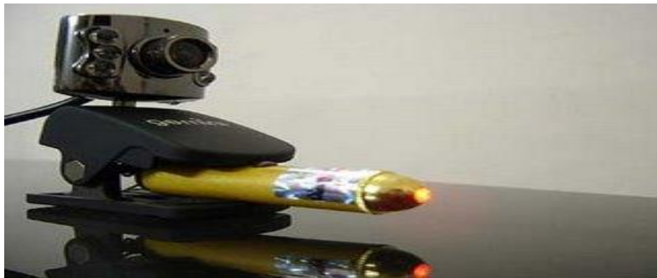
Fig.3 Image capturing device with laser pointer
